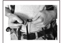
Step 2: Raise the ends of the straps to locate the hook and loops. Insert the hook into an appropriate loop and lower the strap.
