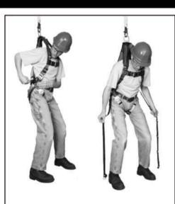
Step 1: Locate and open each case and deploy the suspension straps.
